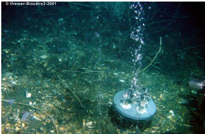
Fig. 11: Bubbles of methane rising through a benthic chamber disposed by the Victor 6000 .
