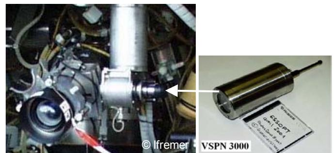
**Fig. 13: *Victor 6000* central pan & tilt unit handles the 3CCD TV with the 4 parallel lasers (left). The future electronic still camera VSPN (right) in its 6000m option will be placed on its right side.**
