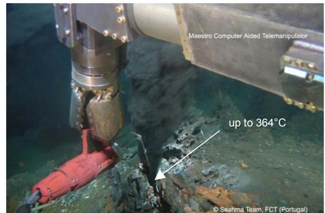
**Fig. 7:** Seahma-1 (2002) cruise: Maestro manipulator operator is performing precise temperature measurements in a black smoker (Rainbow hydrothermal field, venting temperature up to 364°C).
