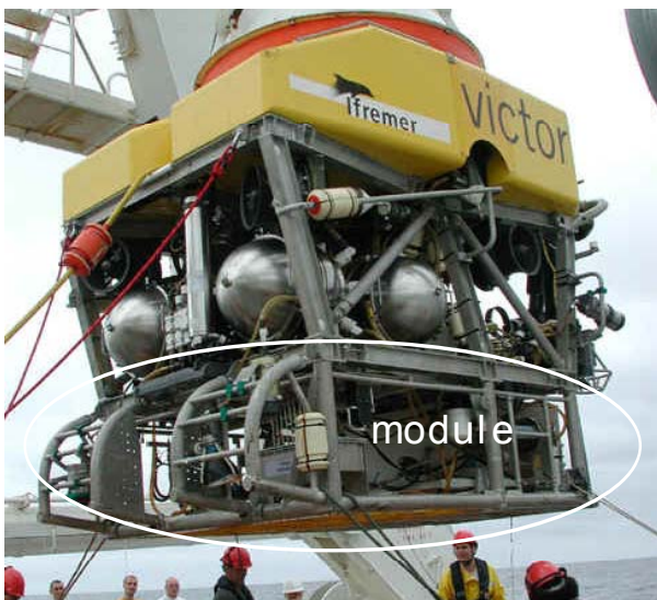
Fig. 2: the 4.6 tons vehicle measuring 3.2 L., 2.2 l., and 2.3 m high includes its large 600 kg sampling module at the inferior part.
