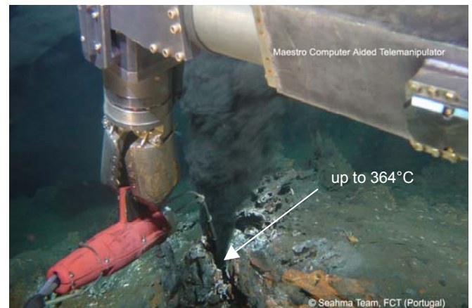
Fig. 7: Seahma-1 (2002) cruise: Maestro manipulator operator is performing precise temperature measurements in a black smoker (Rainbow hydrothermal field, venting temperature up to 364°C).
